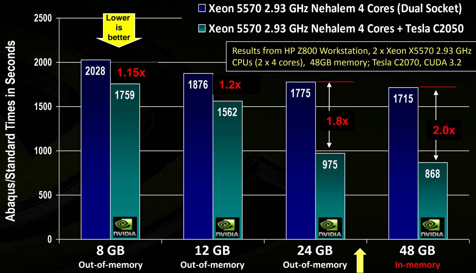
Results from HP Z800 Workstation, 2 x Xeon X5570 2.93 GHz CPUs (2 x 4 cores), 48GB memory; Tesla C2070, CUDA 3.2
